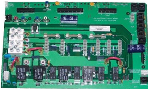
The Relay Board switches 240V to Motors and Heater
